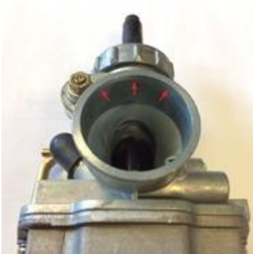
Idle Pilot Jet - Stock Unaltered #32, .0130" No-go
